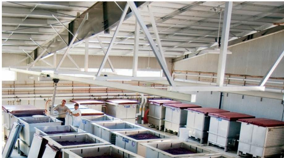
Each portable 3-ton fermenter from Custom Metalcraft holds 750 gallons and is designed with a 1:1 ratio. The rugged tank of 304-stainless steel construction has a sloped bottom and tri-clover fitting for discharge. When the tanks are not in use, they can be stacked and stored with a pallet jack or forklift.
