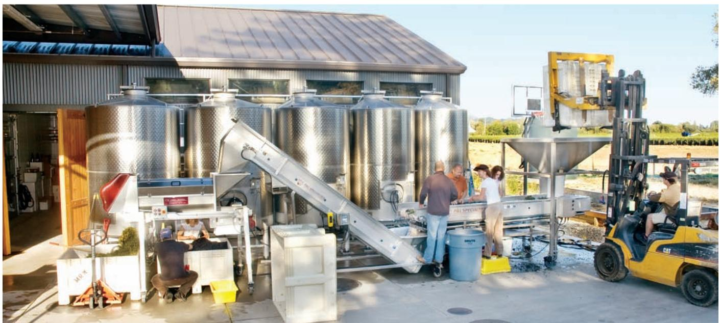
The crush pad with P&L Specialties conveyor and sorting table for careful hand-sorting of grapes. Glycol jacketed blending tanks line the outside wall of the barrel room.
