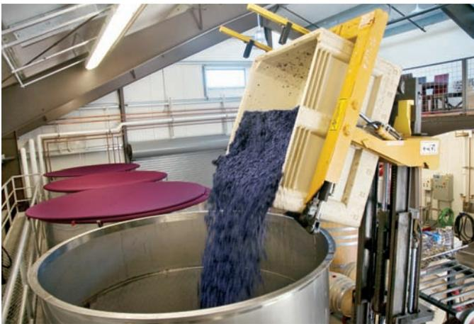
Forklift dumps grapes into one of eight open-top stainless steel fermenters in the 30 foot x 60 foot fermentation room. Natural light enters the room through clerestory windows above the fermentation tanks.
